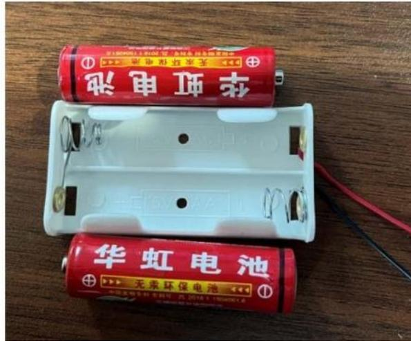
Measure whether the two red and black lines drawn by the battery box have 3V voltage.
