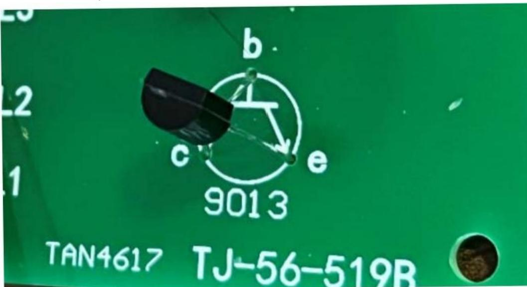
The pin of the triode is defined in the figure below
