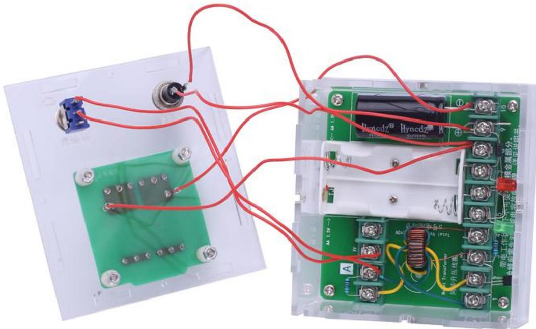
Step 25: Fixed the top acrylic plate by 4pcs M3\*6mm Screw. Note: Install 2pcs brand new AA batteries.
