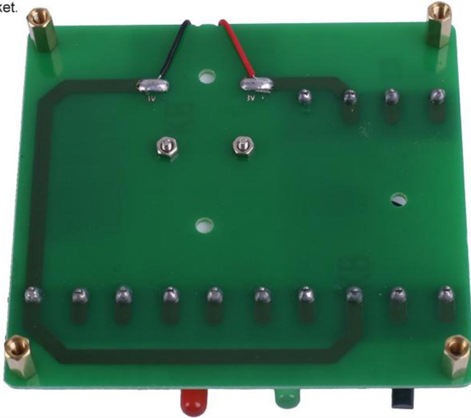
Step 15: Install 2pcs 20cm red wires on Smaller PCB.
