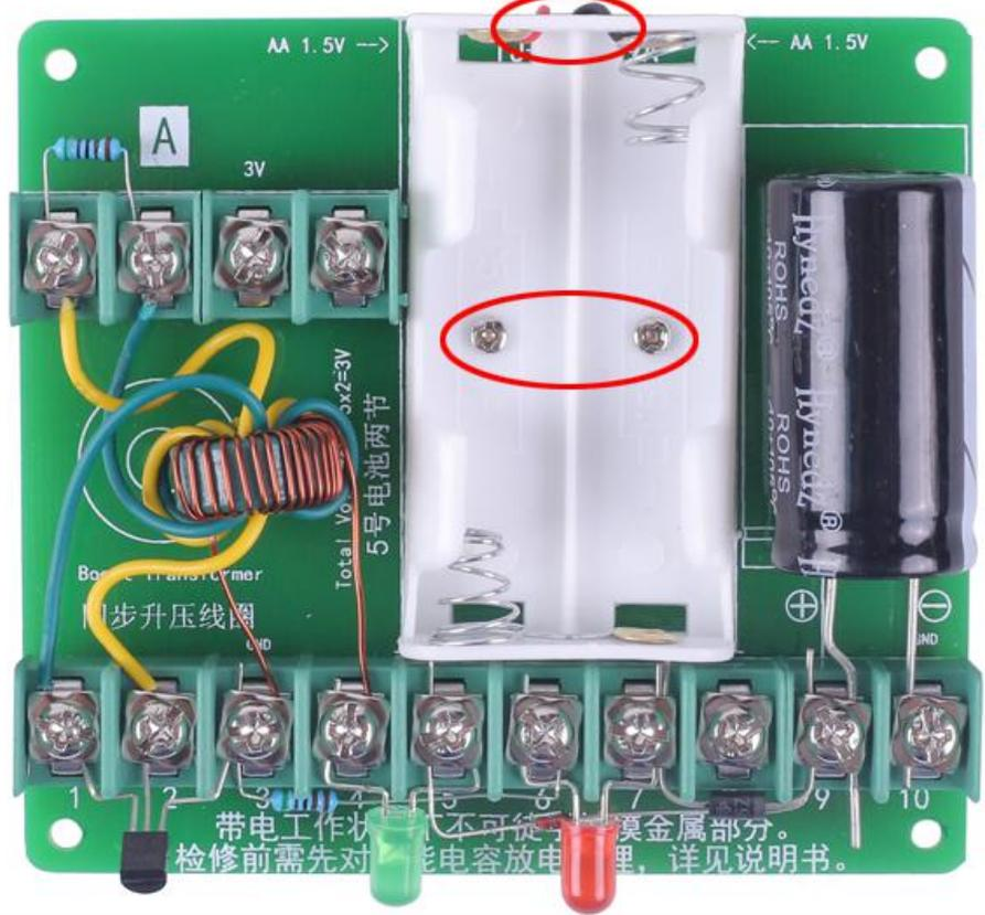
Step 13: Connect power wire form battery box to PCB. Red wire connect to '3V+' and black wire connect to '3V-'. User can cut excess wires.
