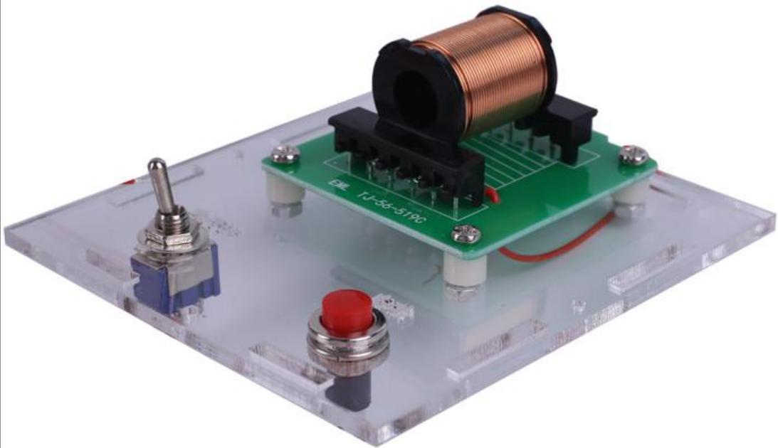
Step 24: Power Switch wires connect to Pin-L2 and Pin-3V;
