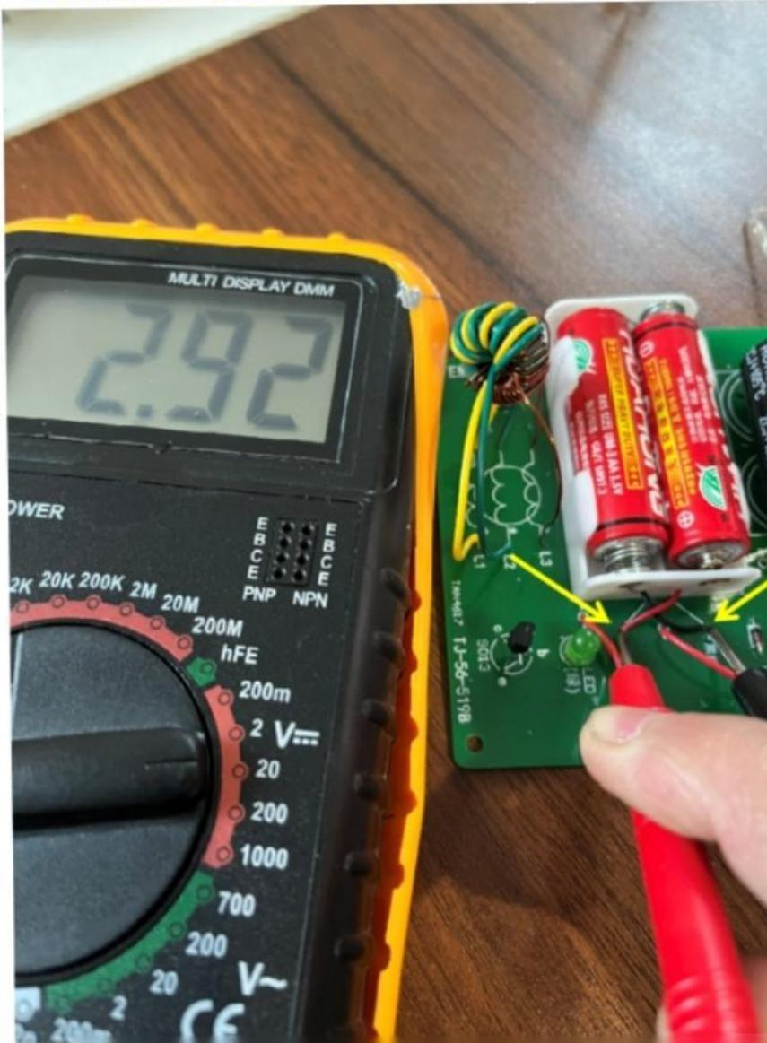
Note that the two red and black lines of the battery case are measured, not the metal contacts on the battery case, so the measurement result is unreliable. As measured in the figure above, 2.92V is the normal voltage. Generally, 2.8–3.2V can be used.
